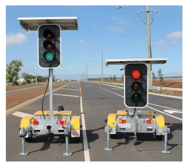
Dual-trailer Portable Traffic Light (PTL) can be towed separately, are solar-powered with maintenance-free batteries for continuous operation. The 200mm aspects use ultra-bright LED's for optimal viewing. The PTL sets maintain constant RF (radio frequency) communication with the each other, as required by Australian Standard AS 4191:2015 for Portable Traffic Signal Systems.
