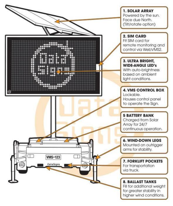
The solar tilt/rotate system developed by Data Signs, allows the operator to tilt and rotate the solar array to the optimal angle and heading to capture the most sunlight each day. By rotating the bottom edge of the solar array to face due north and tilting the solar array slightly for summer and more for the winter season, the amount of sunlight hitting the solar array each day increases and helps keep the batteries charged (subject to environmental conditions).
