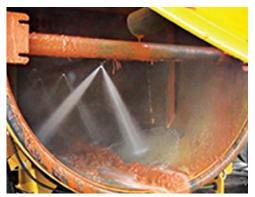
**IN-TANK WASHDOWN SYSTEM.** Saves you cleanup time and makes it easier to remove difficult debris as it delivers a high-pressure water spray to the tank interior while simultaneously dumping material.
