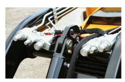
LOW FLOW NEEDED. An optional dual hydraulic auxiliary adds a low-flow option to the hydraulic circuit for use with dual-function attachments.
