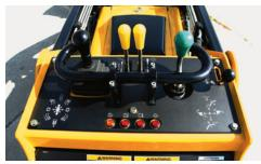
**DRIVABILITY.** Ground drive is controlled by a single, pilot-operated joystick, giving the operator a smooth range of motion, while a single dual-axis joystick controls boom/bucket motion. Warning lights for engine oil pressure, engine temperature and hydraulic oil temperature are located near the controls.
